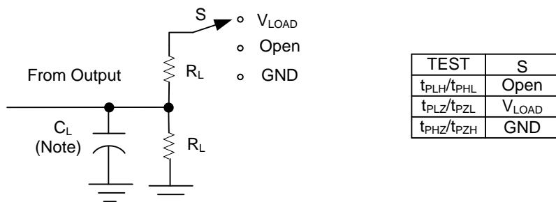
Note:  $C_L$  includes probe and jig capacitance.
