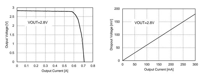
Output Voltage vs Output Current
