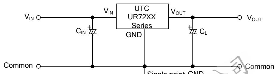
$C_{IN} > 1.0\mu F$  $C_L > 2.2\mu F$  (tantalum capacitor)
