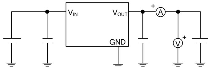
**■ TYPICAL APPLICATION CIRCUIT**
