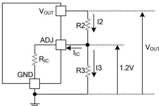
The Output Voltage may be adjustable for any output voltage between its 1.2V reference and its  $V_{DD}$  setting level. An external pair of resistors is required, as shown above.
