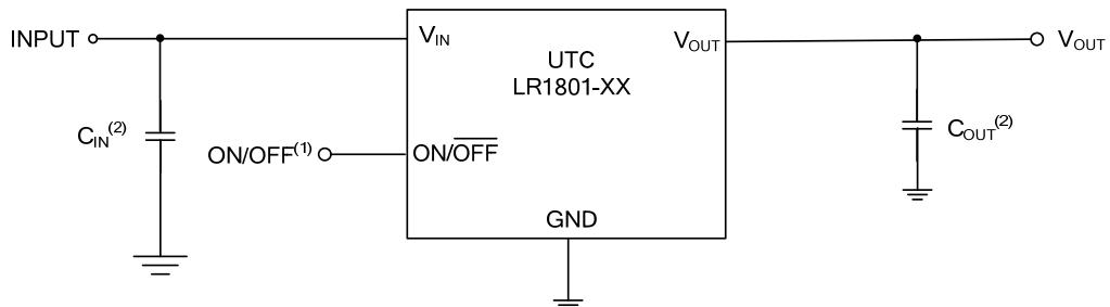
(1) ON/ $\overline{OFF}$  pins must be pulled high through a 10kΩ pull-up resistor.
