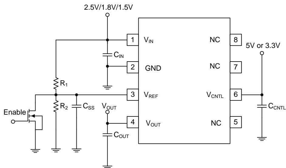
R<sub>1</sub>=R<sub>2</sub>=100KΩ, C<sub>OUT</sub>=10μF(Ceramic)+1000μF under the worst case testing condition
