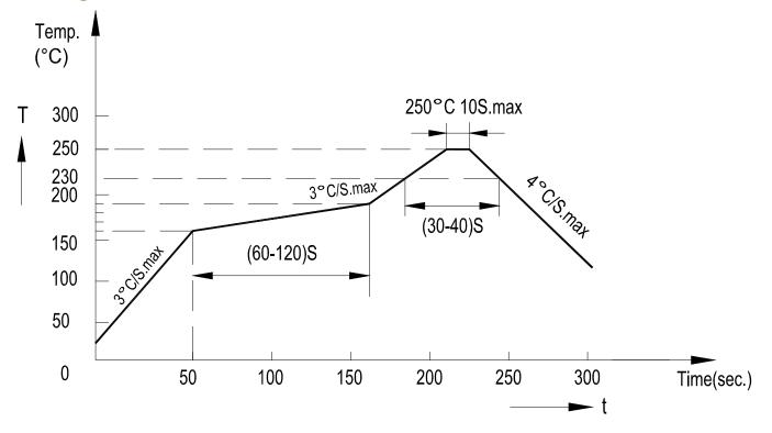
Number of reflow process shall be 2 times or less
