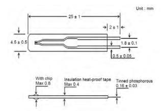
The TJ thermistor possesses ultra thinness of  $500\mu m$  and superior electrical insulation. It is possible to use with safety in ambience where might contact with electrodes.
