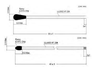
The TA4 thermistor is a high-precision thermal sensing device which is similar to HT thermistor but different with flexible lead-wires.
