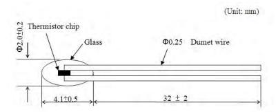
The GS series thermistor is a thermistor sensor with a glass sealed package, which possesses highly reliable and offers a wide operating range of -30  $^{\circ}$ C to 250  $^{\circ}$ C. They can be employed for home electric appliances and high temperature applications.
