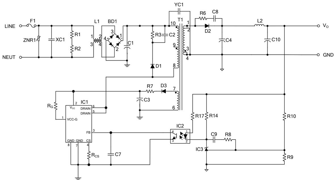
Fig.8 UTC UCS1654S Typical Application Circuit
