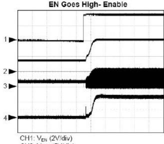
CH2: V<sub>OVP</sub> (5V/div) CH3: V<sub>LX</sub> (10V/div) CH4: I<sub>IN</sub> (500mA/div) Time: 1ms/div
