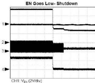
CH2: V<sub>OVP</sub> (5V/div) CH3: V<sub>LX</sub> (10V/div) CH4: I<sub>IN</sub> (500mA/div) Time: 10ms/div
