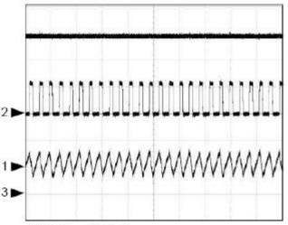
CH1: V<sub>OVP</sub> (2V/div) CH2: V<sub>LX</sub>(10V/div) CH3: I<sub>L</sub> (500mA/div) Time: 2µs/div
