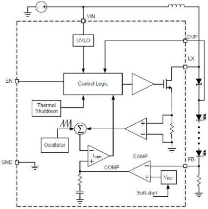
Function Block Diagram of EC4503
