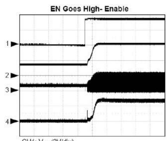
CH1:  $V_{EN}$  (2V/div) CH2:  $V_{OVP}$  (5V/div) CH3:  $V_{LX}$  (10V/div) CH4:  $I_{IN}$  (500mA/div) Time: 1ms/div
