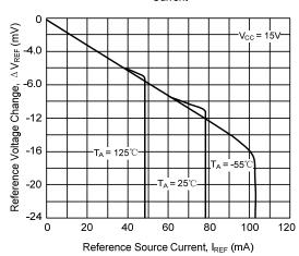
Reference Short Circuit Current vs. Ambient Temperature
