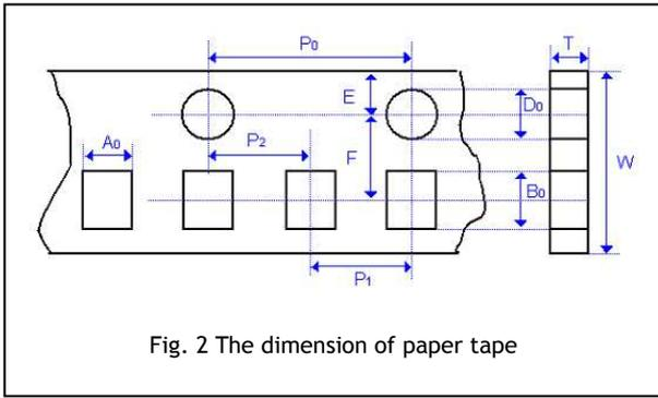
Fig. 2 The dimension of paper tape
