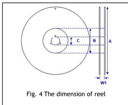
Fig. 4 The dimension of reel
