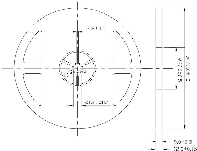
**Note:** Tolerances Unless Dimension  $\pm 0.1\text{mm}$  , Unit = mm
