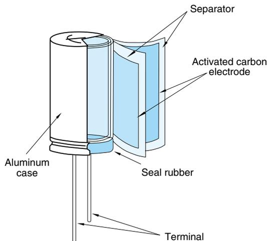
Fig.3 Example of Basic Construction of Cylindrical Cell
