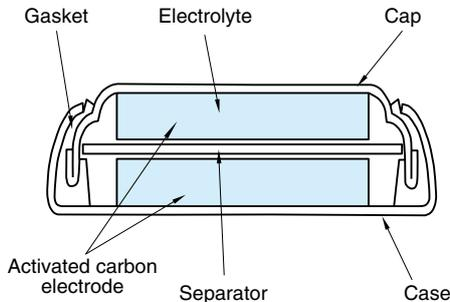
Fig.2 Example of Basic Construction of Coin Cell
