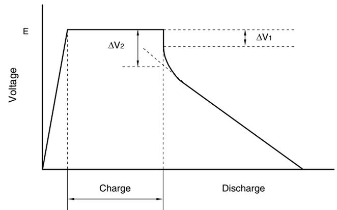
Fig.5 Example of Discharge Curve involving IR Drop
