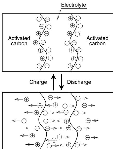
Fig.1 Schematic of Principle of Electric Double Layer Capacitor
