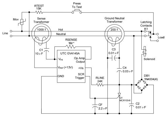
Figure 1. GFI Application Circuit (Three-Wire Outlet)
