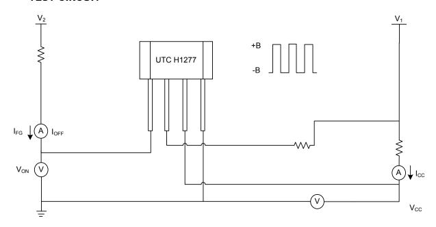
$\label{eq:conditional} \text{Measure V}_{\text{CC}}, I_{\text{CC}} \text{ when DO is off.} \quad \text{Measure V}_{\text{ON}}, I_{\text{FG}} \text{ when FG is on.} \quad \text{Measure I}_{\text{OFF}} \text{ when FG is off.}$
