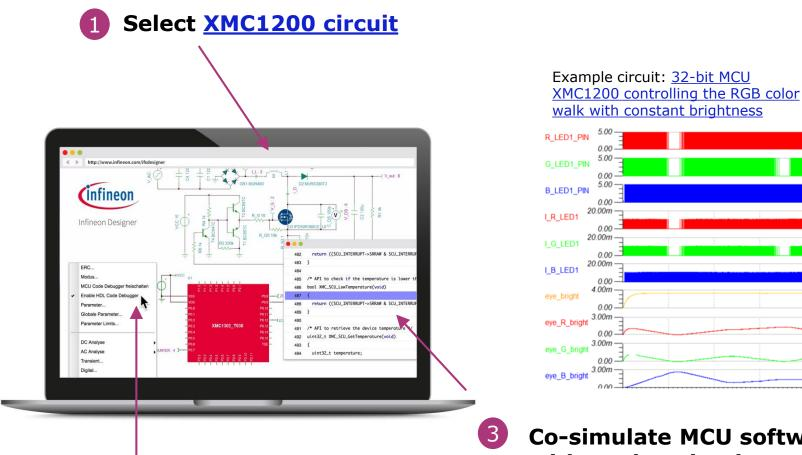
Co-simulate MCU software with analog circuit
