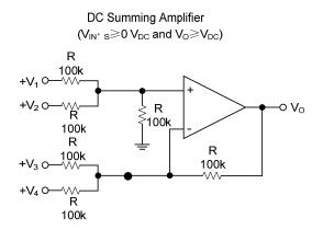
Where:  $V_0=V_1+V_2-V_3-V_4$ ,  $(V_1+V_2) \ge (V_3+V_4)$  to keep  $V_0>0$   $V_{DC}$
