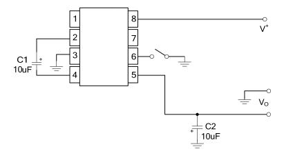
Above figure is the basic application circuit to provide a negative supply from -1.5V  $\sim$  -10V while a positive supply from +1.5V  $\sim$  +10V is available. When V<sup>+</sup>=+5V, the output resistance is about 100 $\Omega$ ; The output voltage is -4V while the load current is 10mA.
