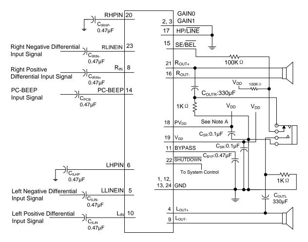
A 0.1- $\mu$ F ceramic capacitor should be placed as close as possible to the IC. A larger electrolytic capacitor of 10  $\mu$ F or greater should be placed near the audio power amplifier for filtering lower frequency noise signals.
