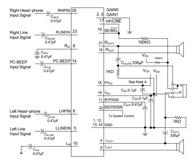
A 0.1- $\mu$ F ceramic capacitor should be placed very close to the IC. A larger electrolytic capacitor of 10  $\mu$ F or greater should be placed near the audio power amplifier for filtering lower frequency noise signals, .
