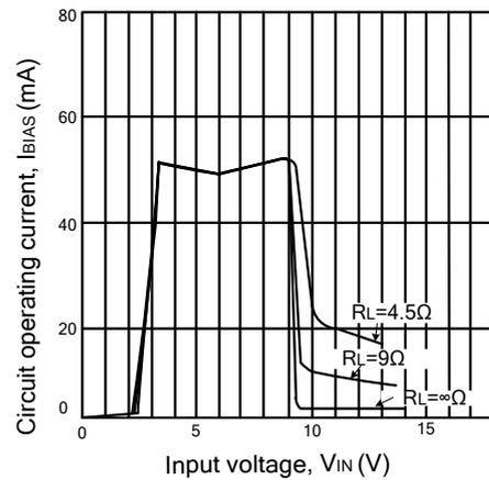
Fig.19 Circuit Operating Current vs .Input Voltage (R12LD20)
