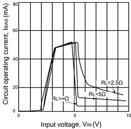
Fig.18 Circuit Operating Current vs .Input Voltage (R09LD20)
