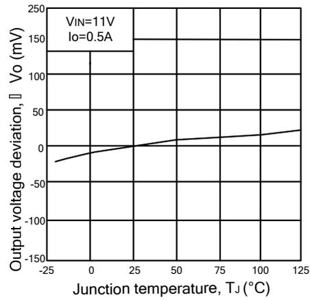
Fig.11 Output Voltage Deviation vs .Junction Temperature (R12LD20)
