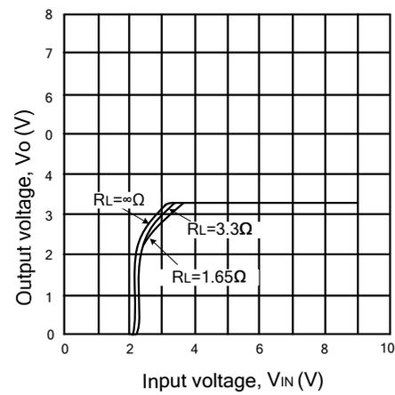
Fig.13 Output Voltage vs .Input Voltage (R05LD20)
