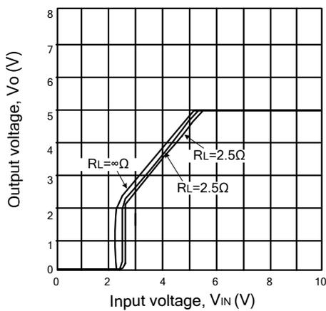
Fig.14 Output Voltage vs .Input Voltage (R09LD20)
