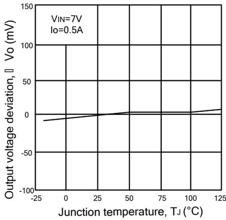
Fig.10 Output Voltage Deviation vs .Junction Temperature (R09LD20)
