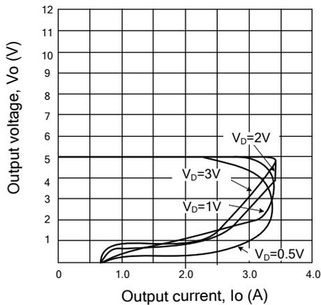
Fig.6 Overcurrent Protection Characteristics (Typical Value)(R09LD20)
