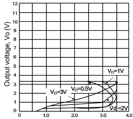
Fig.5 Overcurrent Protection Characteristics (Typical Value)(R05LD20)
