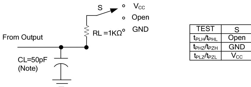
Note:  $C_L$  includes probe and jig capacitance.
