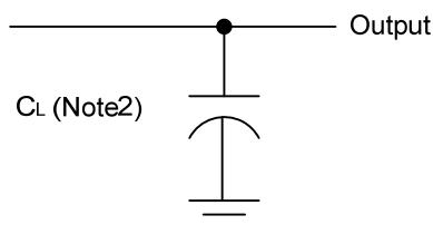
Note 2: CL includes probe and jig capacitance.
