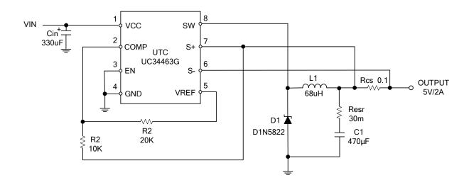
Note: If V<sub>CC</sub>>24V, COMP pin to GND need to add 0.1uF (option) compensation capacitor.
