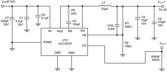
Note: V<sub>OUT</sub>=V<sub>FB</sub>×(1+R1/R2), V<sub>FB</sub>=1.00V, R2 suggest 10k~40KΩ, I<sub>SEN</sub>=3.3A (I<sub>SEN</sub>=V<sub>CS</sub> (0.1V)/RSEN (30mΩ)
