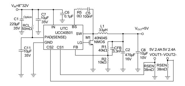
$V_{OUT}=V_{FB} \times (1+R1/R2), V_{FB} = 1.00V, R2 \text{ suggest } 1k^40K\Omega$  $I_{SEN} = 2.63A (I_{SEN}=VCS1(0.1V) / RSEN(38m\Omega))$
