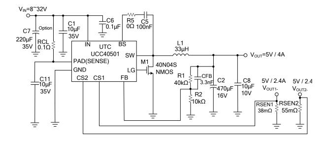
$V_{OUT}=V_{FB} \times (1+R1/R2)$ ,  $V_{FB} = 1.00V$ , R2 suggest  $1k\sim40K\Omega$  $I_{SEN} = 2.63A (I_{SEN} = VCS1(0.1V) / RSEN(38m\Omega))$
