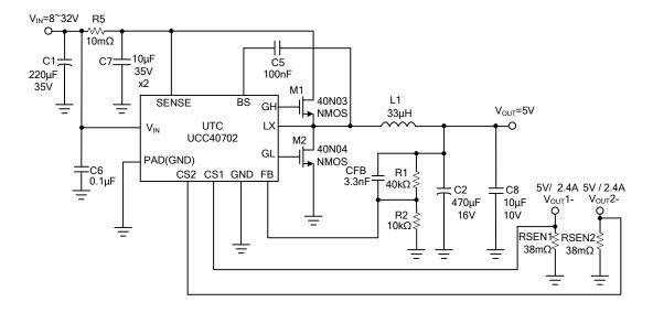
$V_{OUT}=V_{FB} \times (1+R1/R2)$ ,  $V_{FB}=1.00V$ , R2 suggest  $1k^{\sim}30K\Omega$  $I_{SEN} = 2.63A (I_{SEN} = V_{CS}(0.1V) / RSEN(38m\Omega))$
