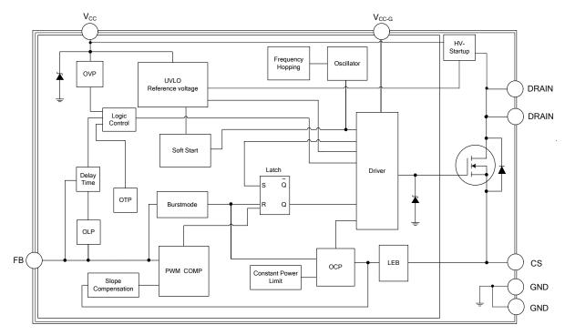
Notes: OLP (Over Load Protection) OVP (Over Voltage Protection) OTP (Over Temperature Protection) OCP (Over Current Protection) UVLO (Under Voltage Latch-Out) LEB (Led Edge Blanking)
