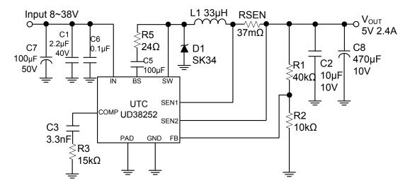
$V_{OUT}$ = $V_{FB} \times (1+R1/R2)$ ,  $V_{FB}$  = 1.00V, R2 suggest 1K~30K $\Omega$  $I_{SEN} = 2.7A (I_{SEN} = V_{SEN}(0.1V) / RSEN(37m\Omega))$
