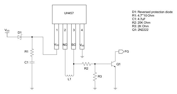
Note: Capacitor C1 is necessary to use for the decoupling between  $V_{DD}$  and  $V_{SS}$  and should be placed as close to the IC as possible.
