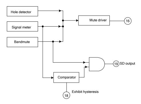
As shown, the SD output is the logical AND of the band mute and S-meter comparator outputs.
