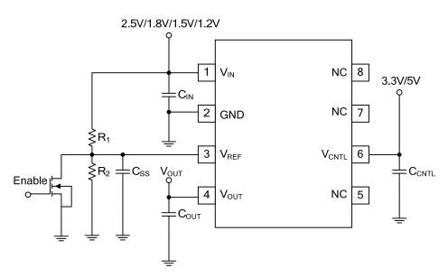
$$\begin{split} R_1 = & R_2 = 1 K \Omega \sim 5 \ K \Omega, \ C_{OUT} = 10 \mu F (Ceramic) under the worst case testing condition \\ C_{SS} = & 0.1 \mu F \ to \ 1 \mu F, \ C_{IN} = 10 \mu F (Low ESR), \ C_{CNT} \\ & V_{REF} = \frac{R_2}{R_1 + R_2} \ V_{IN}(V) \ , \ V_{OUT} \ track \ V_{REF} \end{split}$$
