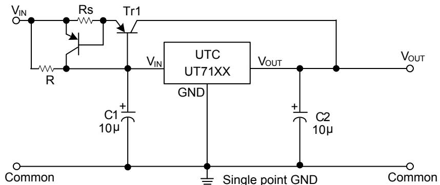
Circuit for increasing output voltage
