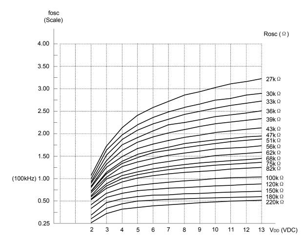
Note: The recommended oscillator frequency is  $f_{OSCD}$  (decoder) $\cong$ 50  $f_{OSCE}$  (UTC UT912E encoder)
