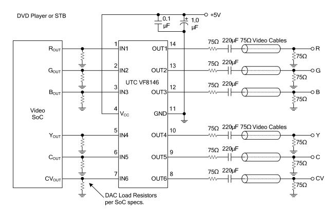
The circuit may be used for direct DC-coupled drive by DACs with an output voltage range of 0V~1.4V. AC-coupled or DC-coupled outputs may be used with AC-coupled outputs, offering slightly lower power dissipation.
